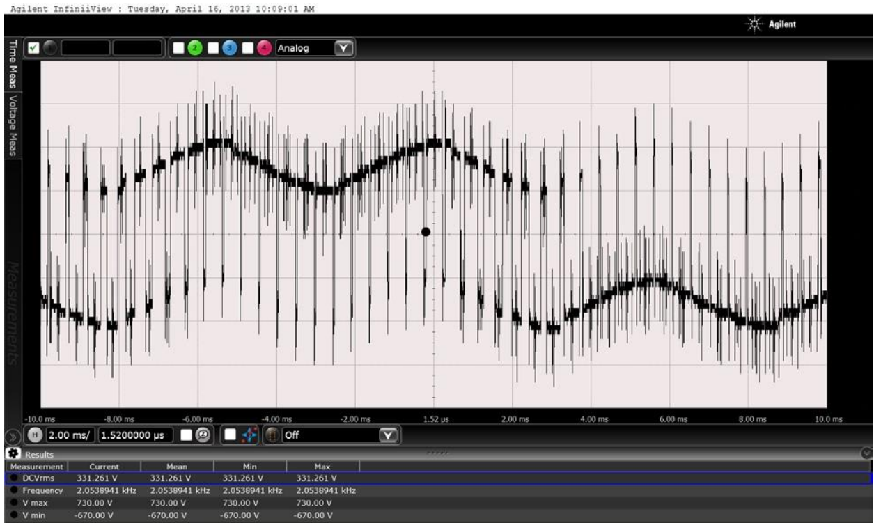
Figure 22: Pump #4 voltage phase to ground, 200 volts per div
