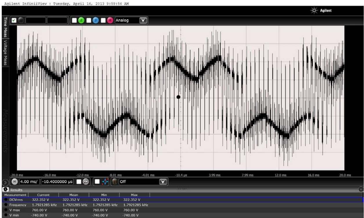
Figure 17: Pump #3 voltage phase to ground, 200 volts per div
