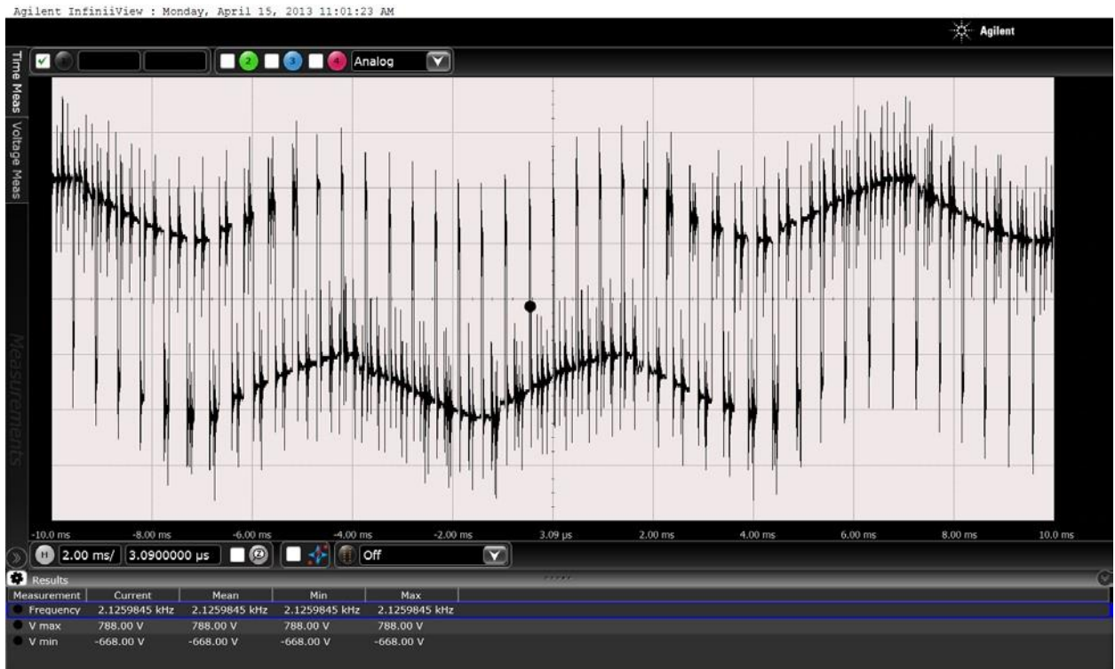
Figure 4: Pump #1 Phase to ground voltage, 200 volts per div
