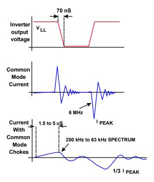
Figure 9 Attenuation of Drive Noise with Common Mode Chokes
