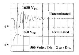
Figure 6 Motor Voltage With and Without Termination Network
