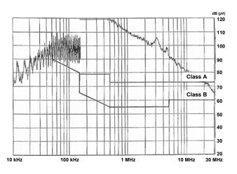
Figure 14 Measurement of Conducted Drive Noise without Filter
