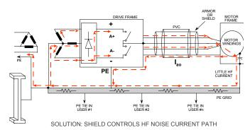
Figure 11 Shielded Power Cable Controls Conducted Noise Path
