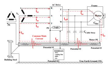
Figure 8 Poor Wiring Practice: Random Unshielded Cable w/o Ground
