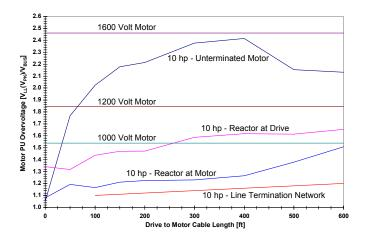
Figure 4 Motor pu Over-Voltage vs. Cable Length vs. Solution
