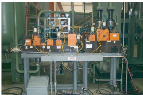
Valve Stand Featuring 2-Way, 3-Way and Check Valves for Flows of 25-1000 GPM
