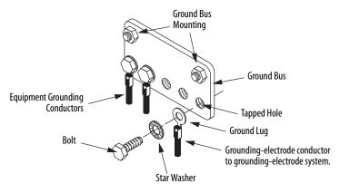
Bonding multiple subpanels creates a common low impedance exit path for the high frequency energy inside the cabinet. Subpanels that are not bonded together may not share a common low impedance path. This difference in impedance may affect networks and other devices that span multiple panels.
