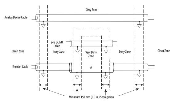
The cable is locally shielded to cross another zone. Each shield is grounded at each boundary and the cable is run close to the panel. The outer shield A is thick-walled steel conduit.
