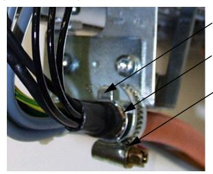
Steel Tab with Turned-up End to Hold Clamp in Place
