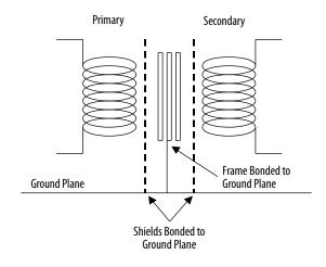
This technique is very effective, though EMC filters are required to meet European regulation standards. Observe these guidelines when installing transformers:
