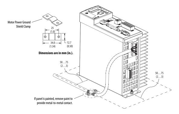
This figure shows an example of wiring with three-phase power and brake wires. The brake wires have a shield braid (shown as gray) that folds back under the cable clamp before the conductors are attached to the motor brake circuit. Thermal switch wires are included in the feedback cable.
