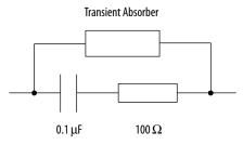
This suppressor across the contact reduces the noise from the wiring inductance as well as the coil inductance.
