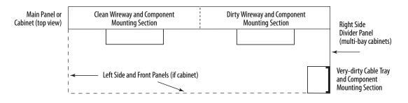
A side panel is fitted on the right to support the power cable shield clamps and any very-dirty wires, cables, or components. This leaves the main panel free for the clean and dirty zones.
